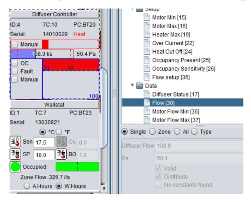
Notice how the airflow volume decreased with a change in control disk position.
