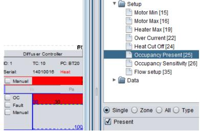
Note: Occupancy present will be selected on all Diffuser controllers that are factory fitted with occupancy sensors.
