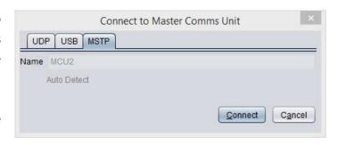
Select the View/Open New Terminal/USB (MSTP) tabs. Press Connect and then 'Show config' to verify the BACnet ID, MAC address and baud rate fields.
